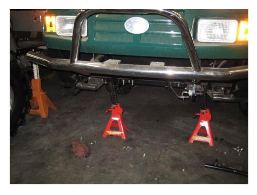
**STEP 2**Place the carrier mount 6 existing OEM bolts on underside of cart and tighten down OEM nylos.
