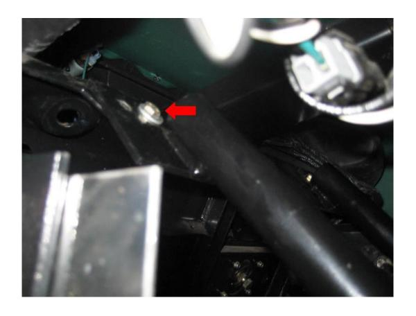
**STEP 6**Go back and tighten all nylocs, on carrier and carrier mounts.
