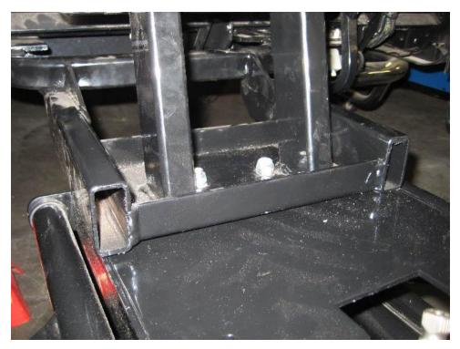
**STEP 4** Place mesh hoop on top of already mounted carrier. Line holes up and place two 1"x3/8" bolts and fasten it together, but DO NOT TIGHTEN YET.
