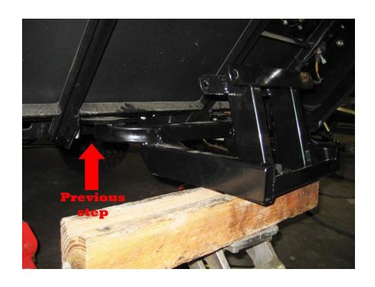
STEP 3 Place carrier under carrier mount installed in step 2. Line up holes and use two 1"x3/8" bolts to fasten together, but DO NOT TIGHTEN YET.
