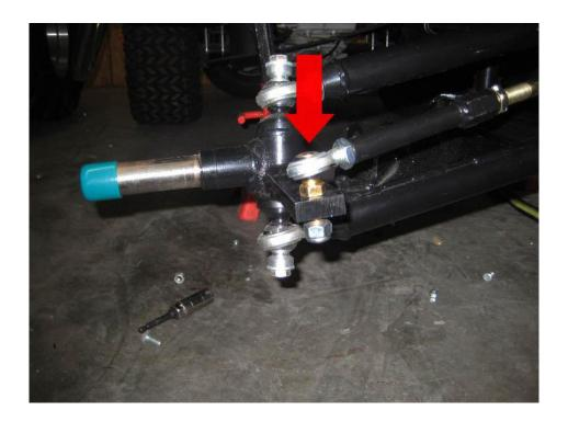
**STEP 8**Place OEM hub over new spindle. Repeat this step for opposite side.
