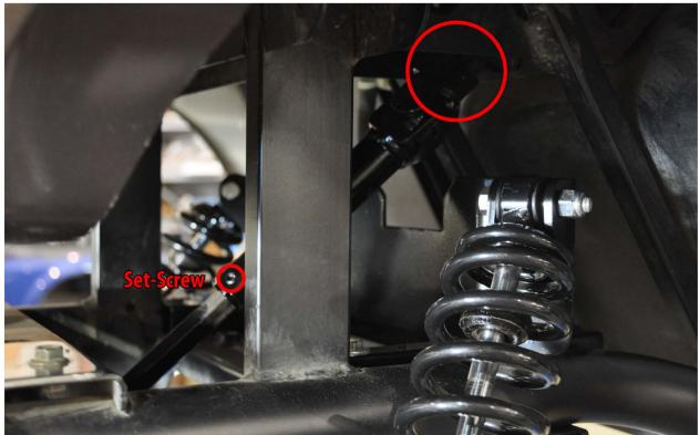
7. Connect the steering linkage to the steering assembly with the intermediate shaft. Loosen the set screw to adjust length accordingly. Retighten set screw when adjustments have been made. Tighten the bolts at each end of the intermediate shaft when in place.
