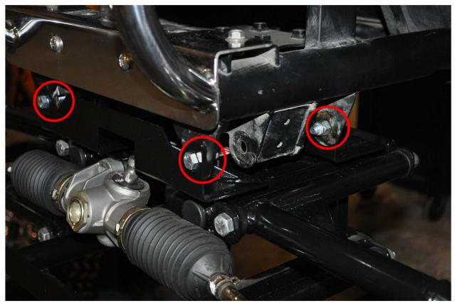
3. Attach the carrier to the chassis using the mounts attached in step 2. Use four 3/8" x 1" and four 3/8" nylocs. With the carrier now mounted to the chassis; tighten the loose bolts from step 2.
