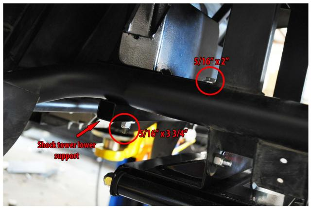
**5A.** Use two 5/16" x 2 bolts, four 5/16" flat washers (top and bottom of frame rails) and two 5/16" nylocs to attach the front of the shock tower to the frame rails.
