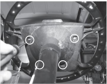
**Step 1:** Remove the 4 philips screws shown and remove the score card holder.
