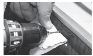
**Step 5:** When drilling or screwing in the dash please use a piece of cardboard to protect the area around the holes from scratches.
