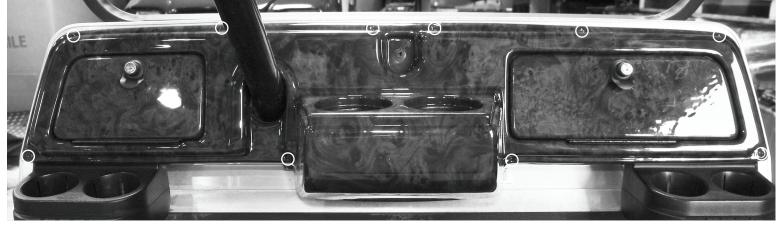
**Step 6:** Slide the dash onto the steering column and line up the dash. The drill points are indentions already made in the dash as shown. Use a long 1/8" drill bit for drilling the holes.
