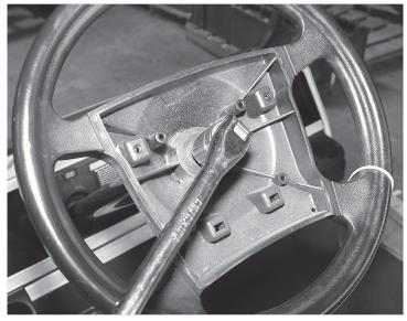
**Step 2:** Loosen the 5/16" nut on the steering column.
