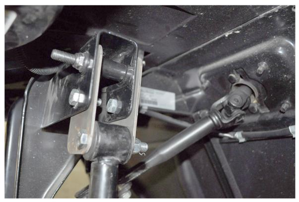
3. Unbolt shock from stock location and re-attach with shock extension plates. Attach plate at top with OEM bolt and nyloc with spacer in-between. Attach mid-section with two 3/8'' x 1'' bolts and nylocs. Attach shock to plate with 3/8'' x 2 1/2'' bolt with nyloc. Tighten hardware. Repeat for opposite side.
