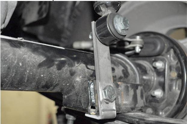
7. Remove shock bottom from axle and install the shock extension brackets. Install bottom of bracket with a 10mm x 40mm bolt and the top of the bracket with a 3/8" x 2" bolt with 3/8" flat washer and 3/8" Nyloc. Tighten allI hardware and repeat on opposite side.
