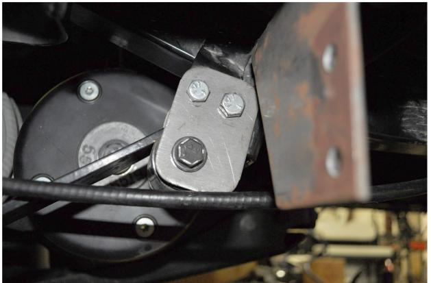
9. Remove front of leaf springs from spring hangers. Install spring hanger extension plates at the front of the leaf springs. Use two plates per side and two 5/16" x 1" bolts and two 3/8" x 1" Bolts with nylocs. Re-attach leaf-spring using OEM bolt and nyloc. Repeat for opposite side and tighten all hardware.
