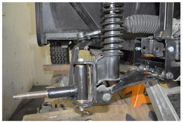
5. Attach new spindles to control arms using included 1/2" x 6" bolts, nylocs and SAE washers. Then attach tie rods to steering arms on spindles using OEM hardware. Tighten hardware and repeat for opposite side.
