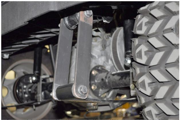
10. Remove stock shackles and replace with new rear shackles using OEM hardware. Tighten all hardware.
