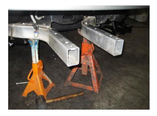
**STEP 2**Slide the new tower over frame rails. Be sure to line up the holes. Push bolts down through tower and frame rails.
