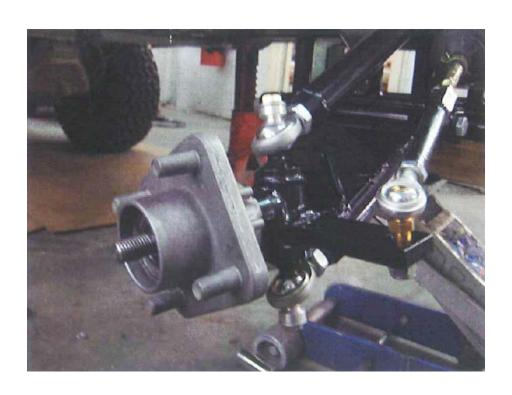
Place new steering shaft on the end of existing steering column. Next attach opposite end to steering rack on the carrier. Tighten both bolts.
