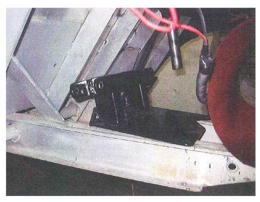
Place already assembled carrier on jack or blocks under frame rails, line up with existing holes.
