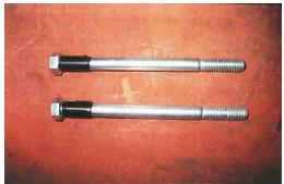
Place two 3/8"x4 1/4" bolts through the carrier, place two spacers over bolts. Next push bolts through the tower plate on top of the frame rails, and place 3/8 nyloc on end.
