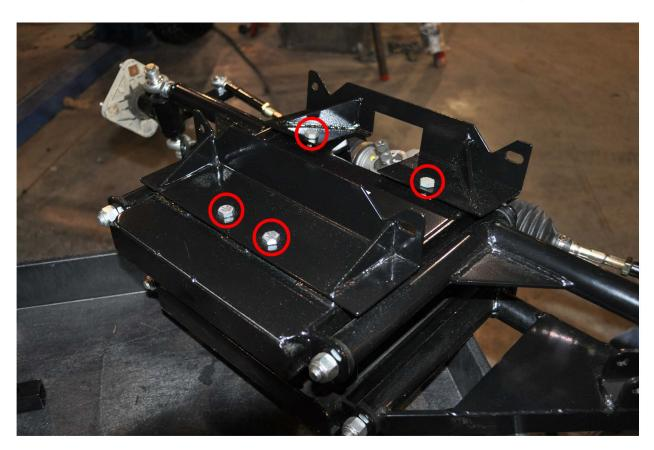
**2.** Attach each of the two included chassis mounts to the carrier using two 3/8" x 1" and two 3/8" nylocs each. (Do not tighten yet.)
