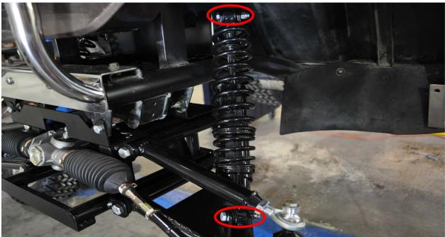
**6.** Mount shocks to the shock tower and lower A-arm using 3/8" x 2" bolts and 3/8" nylocs.
