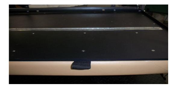
Step 11: Install rear seat cushion to seat deck with eight 1/4" X 1 1/2" screws. Install seat strap between cushion & deck (Fig 11)
