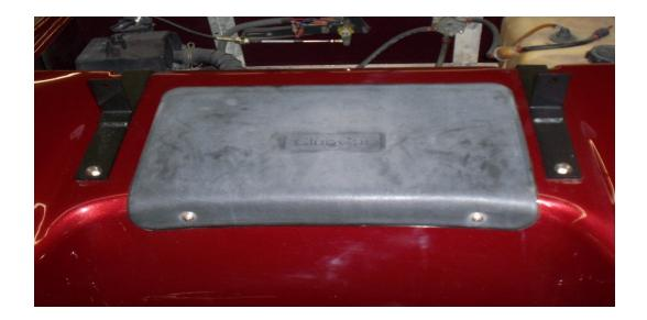
Step 1: Remove OEM Seat back brackets, top supports & rear bumper. Install seat frame supports with 5/16" x 1 1/2" bolts, washers & nyloc nuts. Tighten bolts at this time. (Fig. 1)
