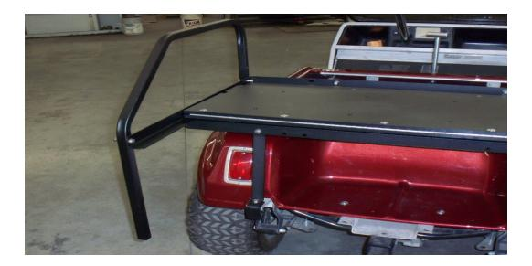
Step 4: Install side rails to seat frame with 5/16" X 1 1/2" bolts, washers, and 2 nyloc nuts & 2 acorn nuts. **Note:** Acorn nuts are installed on rear of side rails (Fig. 4)
