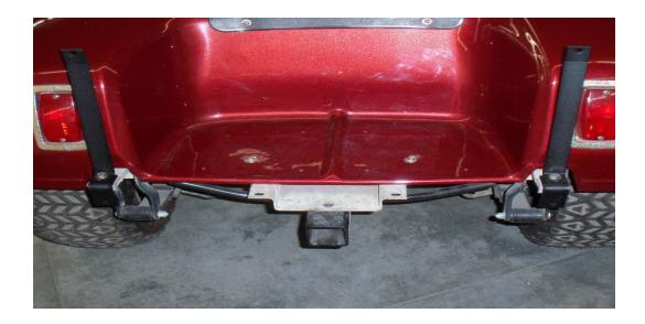
Step 2: Install seat frame supports and step plate brackets to bumper mounts with 5/16" X 1 1/2" bolts, washers, & nyloc nuts. Do not tighten bolts. (Fig.2)
