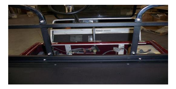
Step 7: Install top supports with 1/4" X 1 3/4" bolts, washers, & nuts (Fig. 7)
