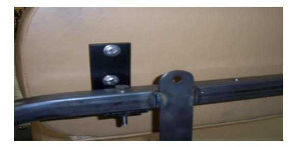
Step 10: Install rear seat back cushion brackets to cushion with 1/4" X 1" bolts & washers. Install cushion to seat frame with 1/4" X 1 3/4" bolts, washers & nuts(Fig.10)
