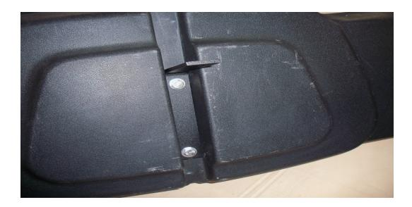
Step 8: Install front seat back cushion brackets with 1/4" X 1" bolts & washers (Fig. 8)
