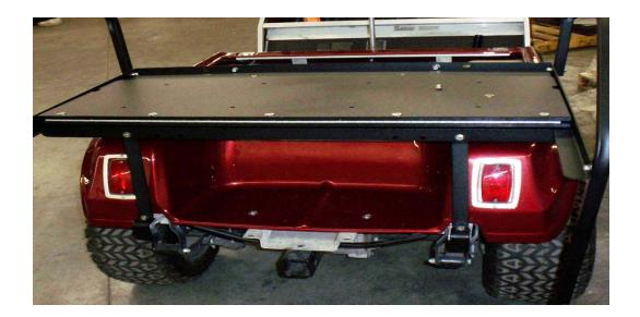
Step 3: Install seat frame with 5/16" X 1" bolts, washers & nyloc nuts (Fig. 3)
