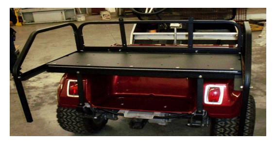
Step 5: Install seat cushion frame with top support brackets facing front of cart with 5/16" X 2 1/2" bolts, washers & nyloc nuts (Fig. 5)
