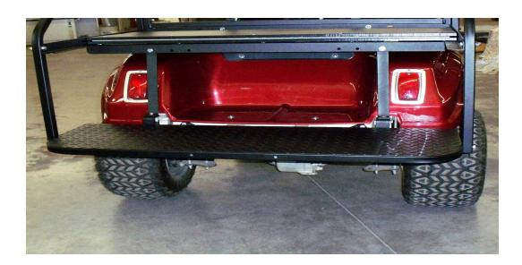
Step 6: Install step plate with 5/16" X 2" bolts, washers & nuts to bumper brackets. Install 5/16" X 2 1/2" bolts, washers, & nuts through side rails. Tighten all Hardware. (Fig. 6)
