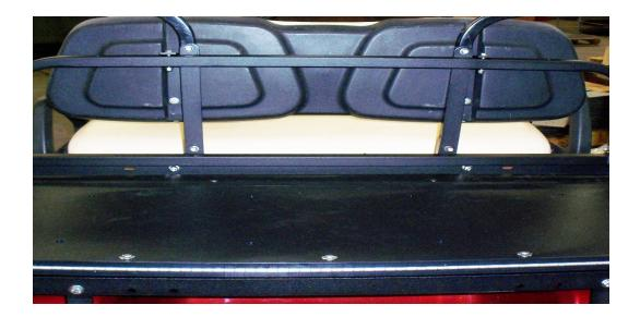
Step 9: Install front seat back cushion to seat frame with 1/4" X 1 3/4" bolts, washers & nuts (Fig. 9)
