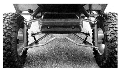
**NOTE:** Apply supplied thread locker to ball joint bolts and tighten bolts. Adjust toe-in with tie-rod (0" - 1/8" toe-in at front of tires).
